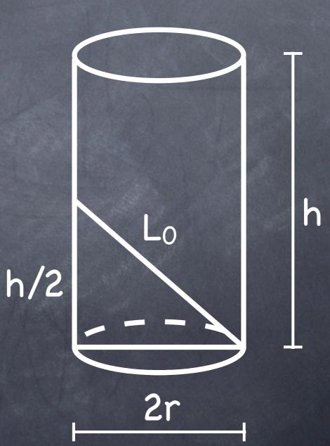
Objective functions:  $V = \pi r^2 h$ . Constraint:  $L_0^2 = (2r)^2 + (h/2)^2$ . Solve for: (A) r (B) r<sup>2</sup> (C) h (D)  $h^2$
