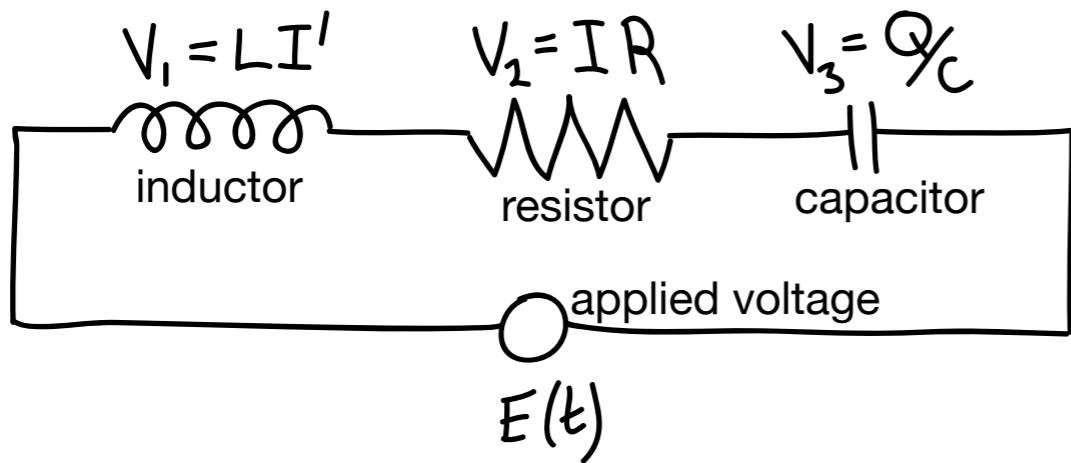
$$\begin{aligned} V_1 + V_2 + V_3 &= E(t) \\ LI' + IR + \frac{1}{C}Q &= E(t) \\ I = Q' & \end{aligned}$$
