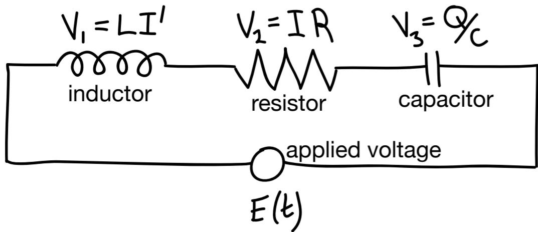
$$V_1 + V_2 + V_3 = E(t)$$
