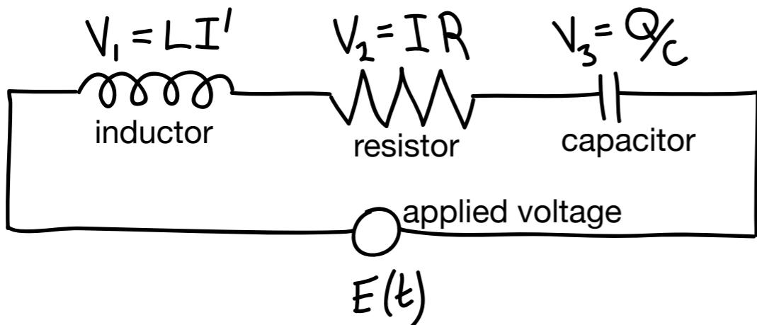
$$V_1 + V_2 + V_3 = E(t)$$
