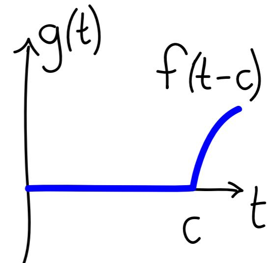
$$\begin{aligned}\mathcal{L}\{k(t)\} &= \int_0^\infty e^{-st} u_c(t) f(t - c) \, dt \\ &= \int_c^\infty e^{-st} f(t - c) \, dt \quad u = t - c, \quad du = dt \\ &= \int_0^\infty e^{-s(u+c)} f(u) \, du \\ &= e^{-sc} \int_0^\infty e^{-su} f(u) \, du \quad = e^{-sc} F(s)\end{aligned}$$
