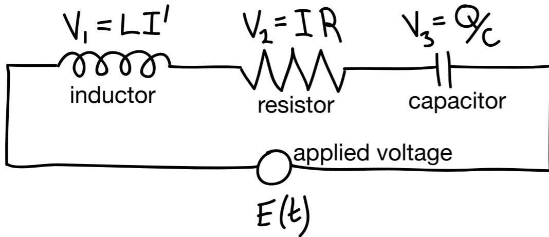
$$V_1 + V_2 + V_3 = E(t)$$
