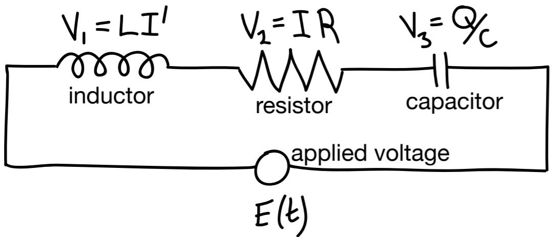
$$V_1 + V_2 + V_3 = E(t)$$
