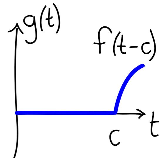
$$\begin{aligned}\mathcal{L}\{k(t)\} &= \int_0^\infty e^{-st} u_c(t) f(t - c) \, dt \\ &= \int_c^\infty e^{-st} f(t - c) \, dt \quad u = t - c, \quad du = dt \\ &= \int_0^\infty e^{-s(u+c)} f(u) \, du \\ &= e^{-sc} \int_0^\infty e^{-su} f(u) \, du\end{aligned}$$
