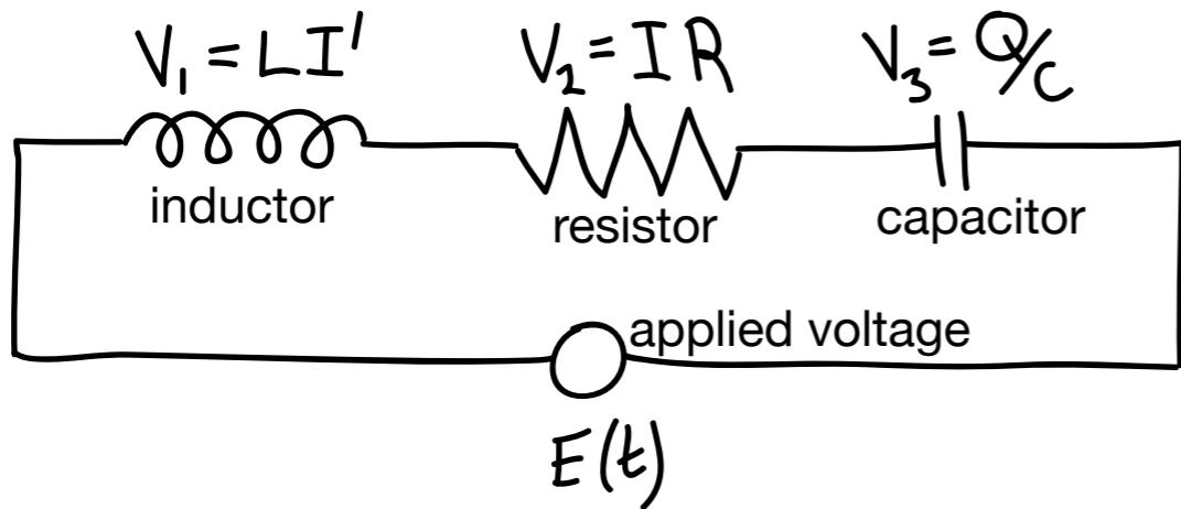
$$\begin{aligned} V_1 + V_2 + V_3 &= E(t) \\ LI' + IR + \frac{1}{C}Q &= E(t) \\ I = Q' & \\ LQ'' + RQ' + \frac{1}{C}Q &= E(t) \end{aligned}$$
