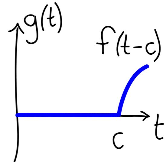
$$\begin{aligned}\mathcal{L}\{k(t)\} &= \int_0^\infty e^{-st} u_c(t) f(t - c) \, dt \\ &= \int_c^\infty e^{-st} f(t - c) \, dt \quad u = t - c, \quad du = dt \\ &= \int_0^\infty e^{-s(u+c)} f(u) \, du\end{aligned}$$
