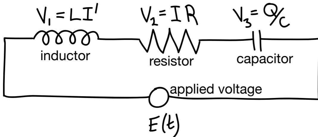
$$V_1 + V_2 + V_3 = E(t)$$
